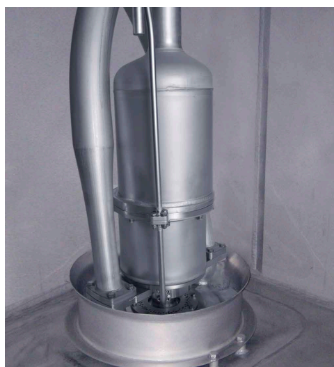
Framo cargo pump in tank
