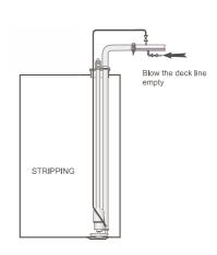
Avoid dry-running of the cargo pumps during tank cleaning.
