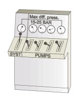
7. It is recommended to operate several cargo pumps, each at reduced capacity, to meet the required pumping rate.
