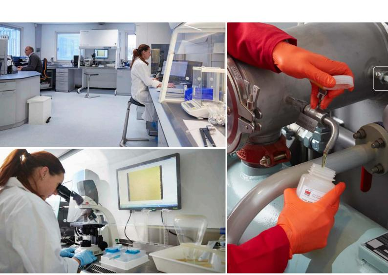
A Framo hydraulic oil sampling kit is supplied, including sampling bottles and instructions. Send an oil sample to one of our laboratories according to the inspection and analysis plan, available on MyPage, your online platform, providing quick access and an overview of Framo-related services and activities.
